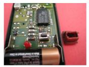
3. Remove old rubber button from electronic switch lifting it up gently with tip of the finger.
