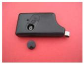
4. Press fit new Silicone button in till it engages with the hard shell of remote.
