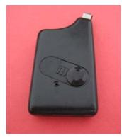
5. Once button fitted in put remote together in reverse order. Close both parts of the shell and srew it together.
